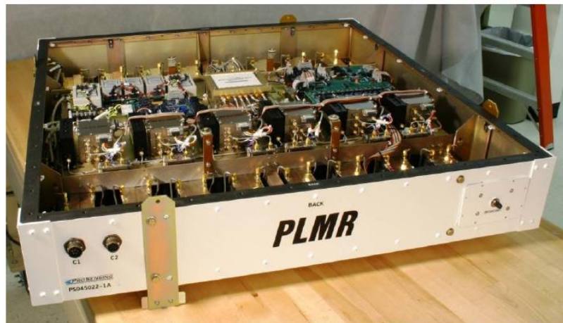
Figure 3-3. View of PLMR with the cover off.
