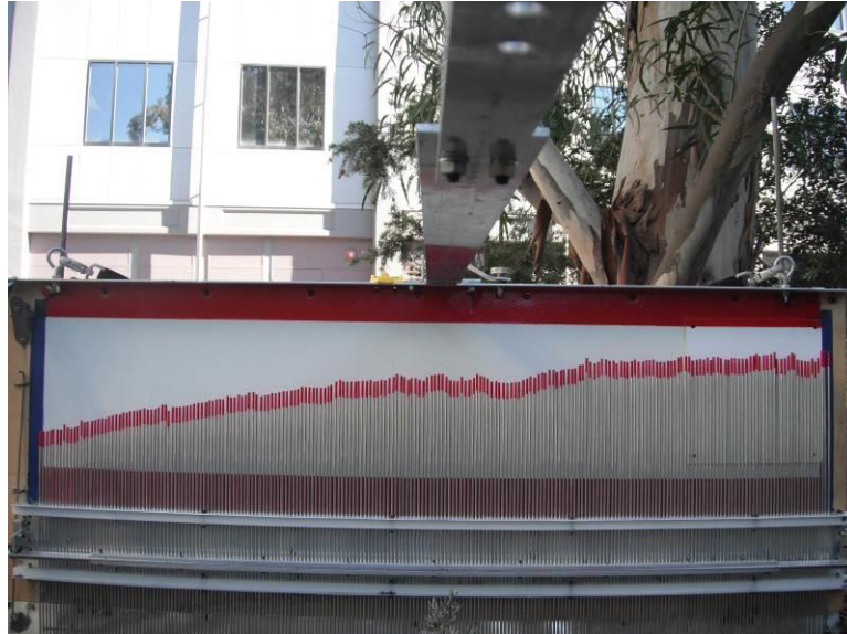
Figure 7-4. Pin profiler for surface roughness measurements.
